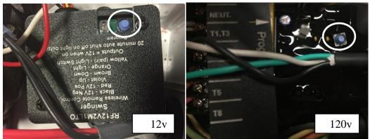
With power on push and hold the small blue "program" button until the red light comes on. On your remote, press and release any button; The red light will blink once. If you have multiple remotes, move to the next one, press a button, the red light will blink twice, continue will all remotes. Once all remotes have been programmed, the red light will go out after 5 seconds. Your remote transmitters are ready for use.
