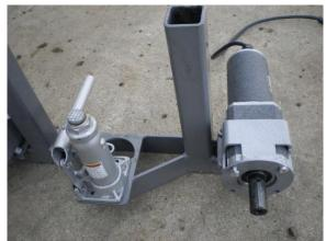
Next slide the wheels onto the motor shaft with the valve stem out. Secure in place using the 3/8 X 3/4" cap screw, lockwasher, and large flat washer.
