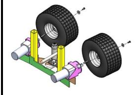
After removing the tape, slide each wheel on to the motor shaft with the valve stem out, securing with the 3/4" Flange bolt and fender washer. Adding a coat of anti-seize to each
